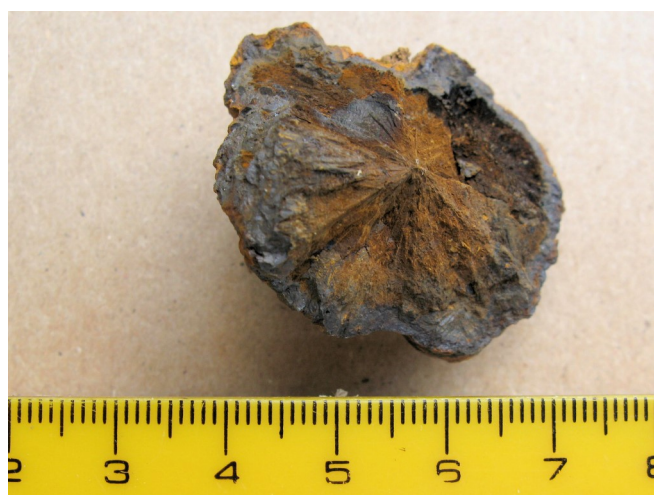
Fig. 3 Fractured pyrites surface showing radial lines
